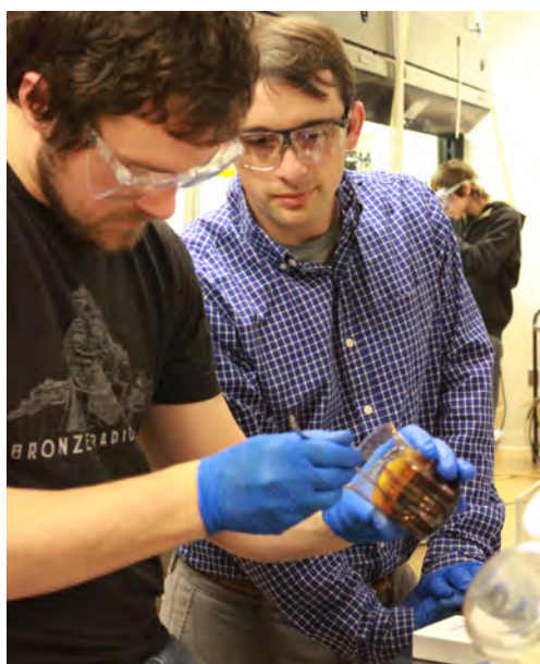
Chemistry professor Troy Townsend '07 (right) with student Keene Kelderman '15 prepare reagents for inorganic nanocrystal synthesis reactions. At left, a spray-on nanocrystal solar cell array.
